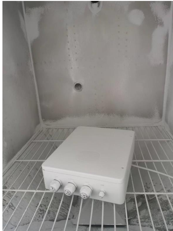
Test setup of IP6X
