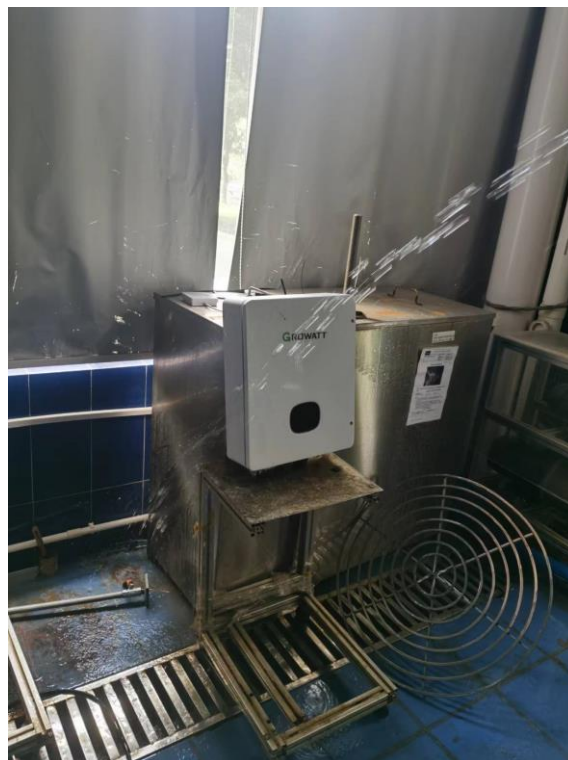
Test setup of IPX5
